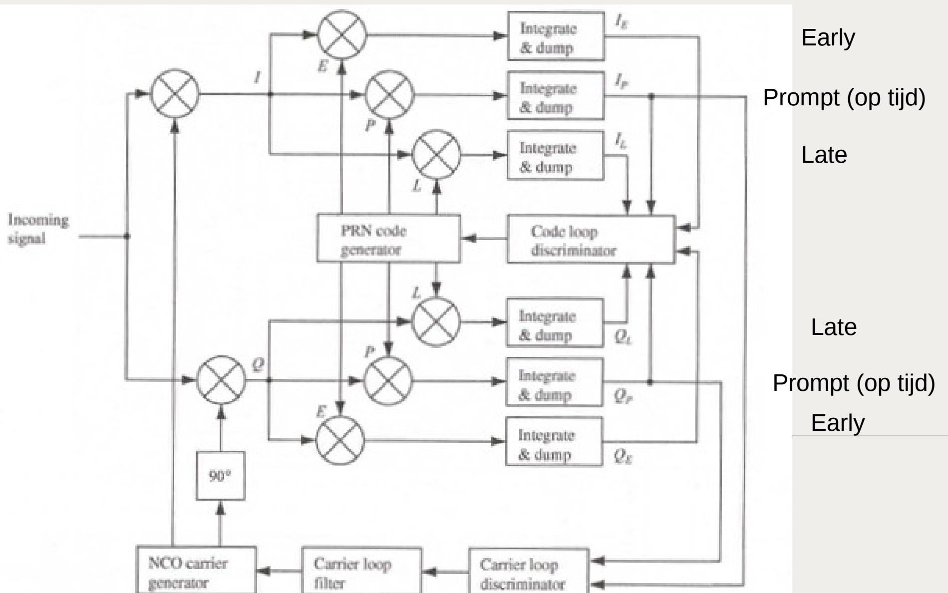
FIGURE 7.20. The block diagram of a complete tracking channel on the GPS receiver.
