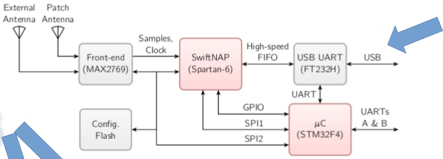
Figure 2: Piksi Block Diagram
