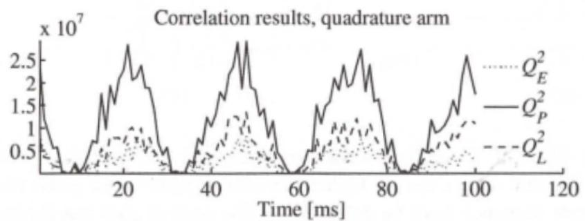
FIGURE 7.13. Output of the six correlators in the in-phase and quadrature arms of the tracking loop. Acquisition frequency offset is 20 Hz and PLL noise bandwidth is 15 Hz (for demonstration purpose).
