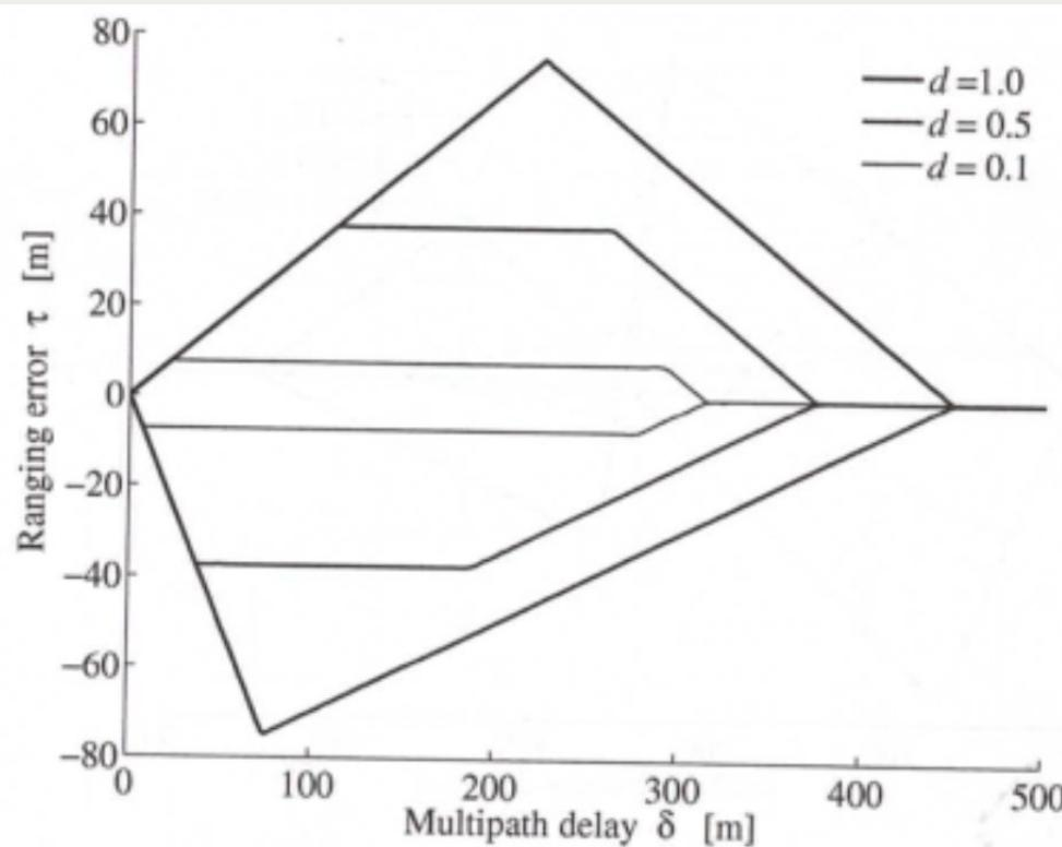
FIGURE 7.17. Multipath error envelope for noncoherent early/late detector for C/A code,  $\alpha = 0.5$ . The positive multipath error corresponds to constructive interference while negative multipath error corresponds to destructive interference.
