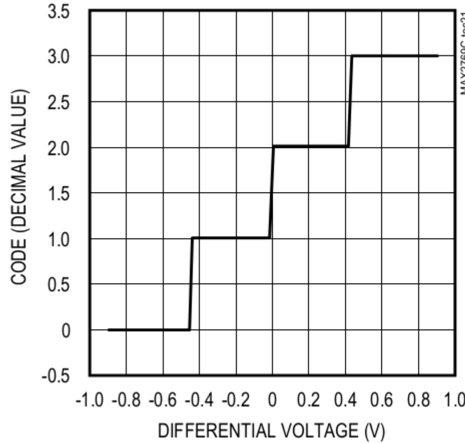
3-BIT ADC TRANSFER CURVE
