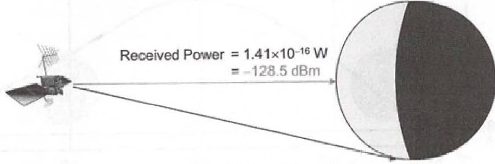
$$\text{Received Power} = 1.41 \times 10^{-16} \text{ W} \\ = -128.5 \text{ dBm}$$
