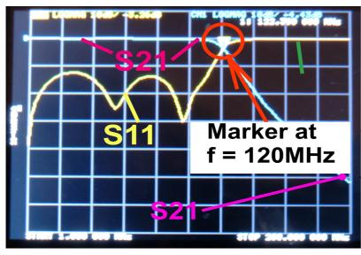
Note: The frequency marker can be moved using the MFS rocker action either left or right. All the data is shown at the top of the screen.
