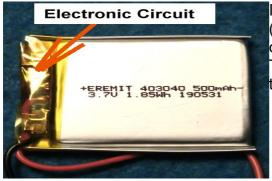
I have ordered one of these batteries on The Internet (6 Euros) and discovered that it contains a tiny circuit board.
