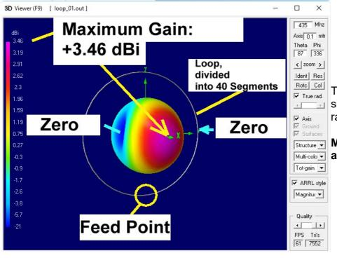
This is a 4NEC2 simulation of the 3D radiation pattern.
