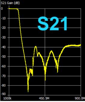
**S21** decreases after leaving the pass band down to -80 dB. But even up to 900 MHz the maximum value is -38 dB (= minimum stop band attenuation)
