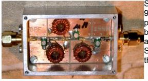
Since the current calibration is from 50kHz to 900MHz this is a good object to measure. The picture shows the test piece. It is a printed circuit board with SMA connectors attached using right angle copper sheets. The inner conductors of the SMA connectors form a low reflection connection on the central microstrip.
