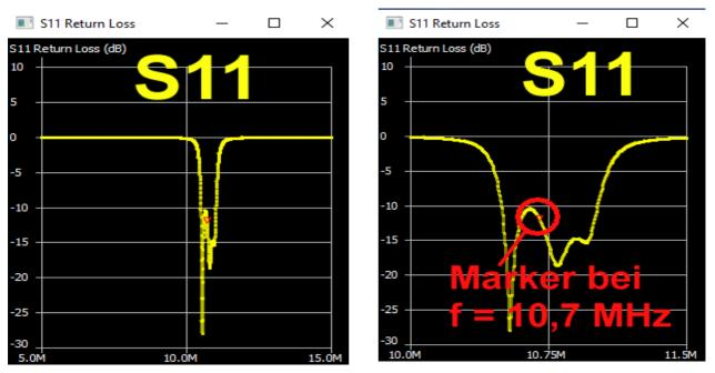
The left illustration uses a frequency range from **5....15 MHz**, the right one from **10...11.5 MHz**
