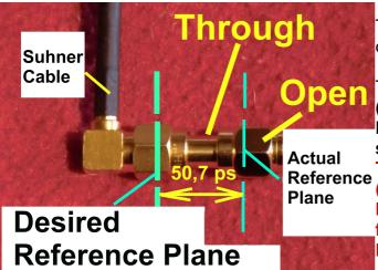
This is the hardware setup for the OPEN calibrating process:
