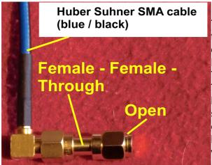
This opens a list that starts with OPEN. Attach the SMA OPEN calibration standard to the end of the cable connected to CH0 using the Female to Female coupler.
