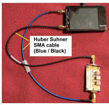
The solution is to purchase two very high quality cables (Huber Suhner with blue black outer), these are specified up to 18GHz. They should remain permanently attached to the NanoVNA having been fitted using an SMA torque wrench purchased from The Internet. If that is done the reproducibility of the calibration for S11 will only have a deviation up to 0.1....0.2dB.
