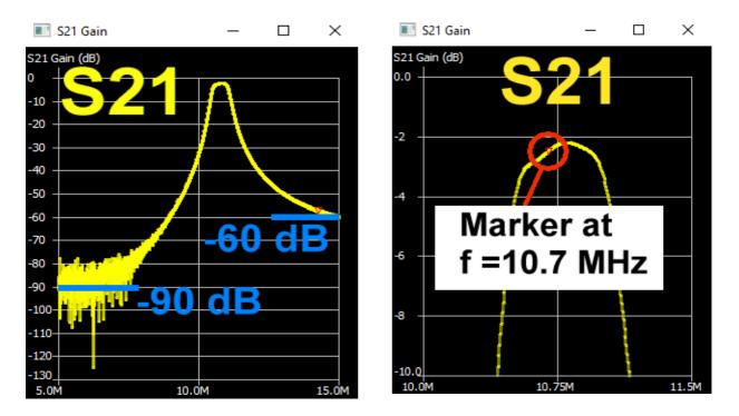
The left illustration shows a remarkable **stop band attenuation of -90 dB for f = 5 MHz** and **-60 dB for 15 MHz**.
