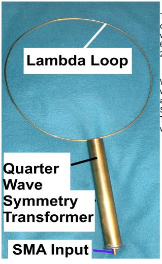
This antenna consists of a wire with a diameter of 2mm and a length equal to the wavelength of a signal with f = 433 MHz (I = 693 mm). The wire forms a circle (diameter = 220 mm).
