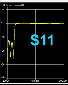
This is **S11 for the 50kHz to 900 MHz frequency** range. The passband can be identified without any efforts (= low reflection) and in the stop band we get a total reflection with **S11 = 0** dB
