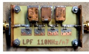
The SMA sockets are solded to two bended copper sheets. Thus the central conductor of the socket touches the central Microstrip Line and is then solded. This gives a transition with low reflection.
