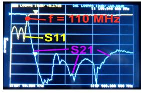
As soon as the measuring cables are connected to the test piece this picture appears.
