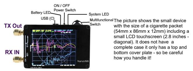
On the left there are of two SMA sockets: the RF input and output. The upper socket is the transmit port (CH0) and is the channel for S11 measurements (reflection). The lower socket is the receive input (CH1) and used for transmission measurements (S21).
