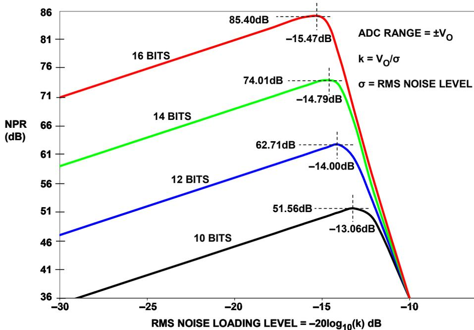
**Figure 2: Theoretical NPR for 10, 12, 14, and 16-bit ADCs**
