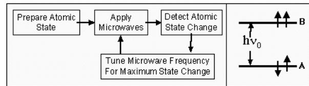
Figure 4: Generalized Atomic Resonator [1]
