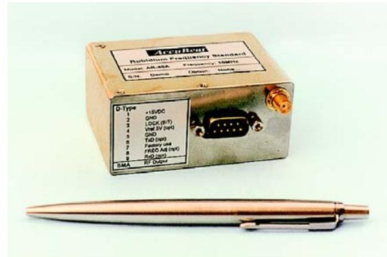
Figure 9: Rb Frequency Standard, Model AR-40A
