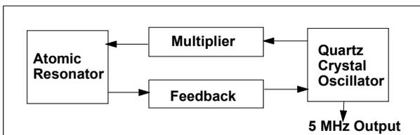
Figure 3: Block Diagram of an Atomic Freq. Std. [1]
