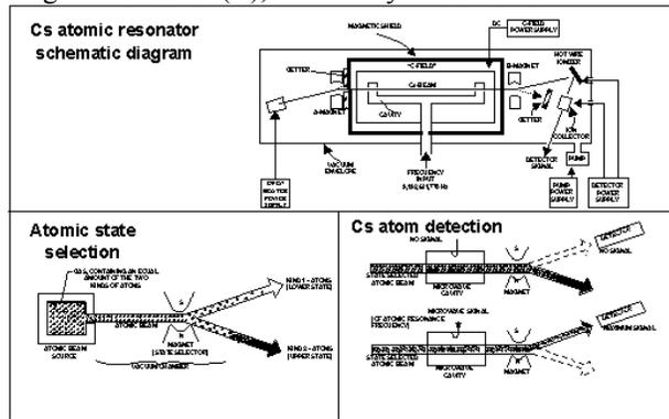
Fig. 5: Cs-Beam Freq. Std. General Block Diag. [1]
