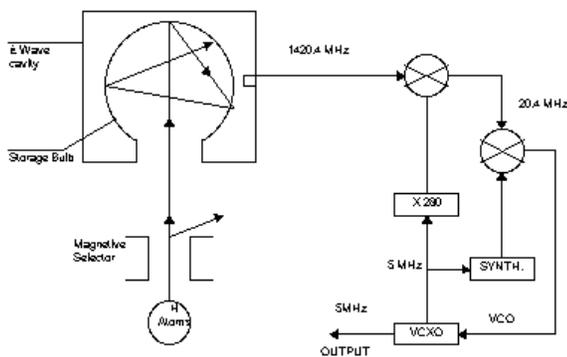
Figure 7: Active Hydrogen Maser Schematic
