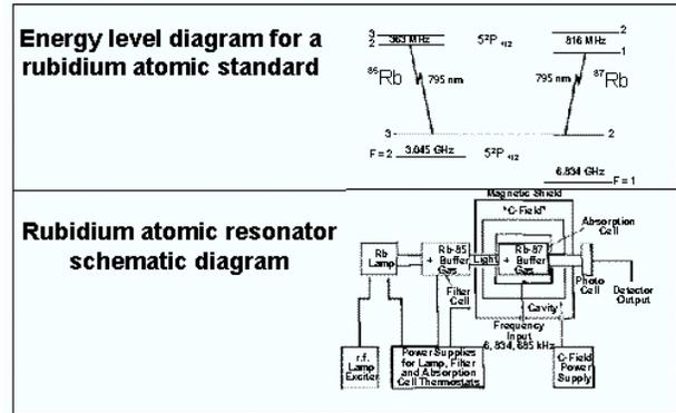
Fig. 6: Rb Frequency Std. General Block Diag. [1]
